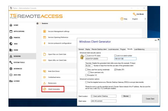
It enables you to create 2 types of connection clients which can be copied to the users' Desktop or onto a USB stick for portable use.
