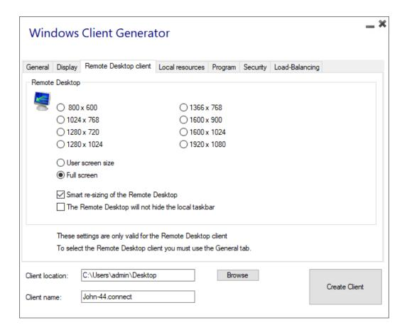
You can check the boxes to enable smart-sizing of the Remote Desktop, and if you want the Remote Desktop not to hide or overlap the local taskbar.
